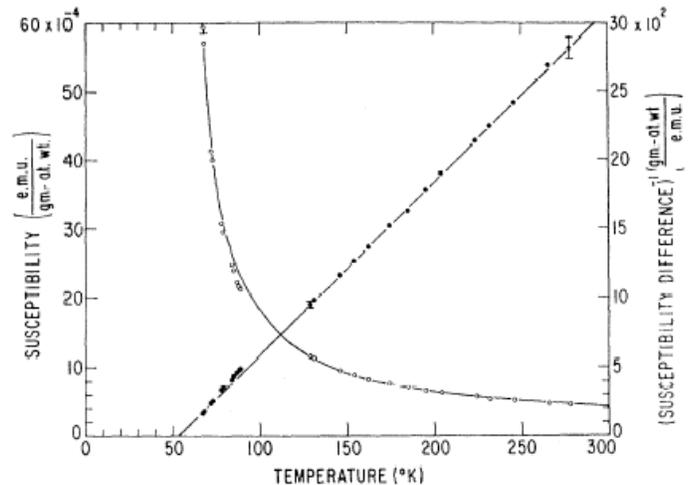
FIG. 3. Susceptibility (open points) and reciprocal susceptibility difference  $(\chi - \chi_0)^{-1}$  (solid points) for sample No. 5(1) showing the Curie-Weiss behavior above the transition temperature.
