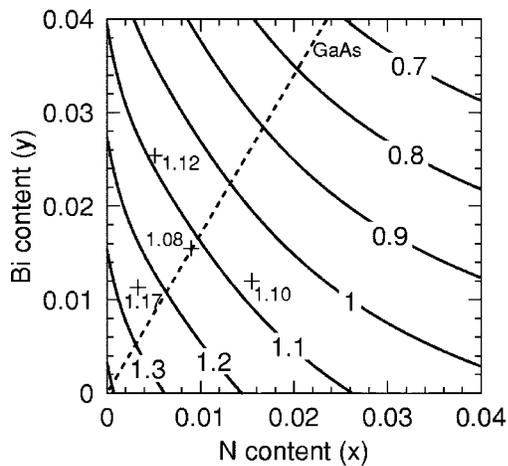
FIG. 4. Band gap map for strained  $\text{GaN}_x\text{As}_{1-x-y}\text{Bi}_y$  on GaAs substrate using Eq. (1) with  $\gamma=0.7\pm 0.7\text{ eV}^{-1}$ . Contours and experimental data points (+ symbols) are labeled in eV. The lattice matched condition to GaAs is shown by the dashed line.
