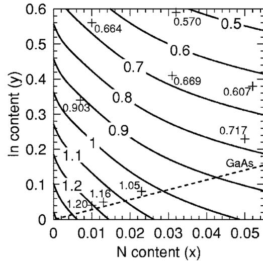
FIG. 3. Band gap map for strained  $\text{Ga}_{1-y}\text{In}_y\text{N}_x\text{As}_{1-x}$  on GaAs substrates calculated from Eq. (1) with  $\gamma = -0.47 \pm 0.10 \text{ eV}^{-1}$ . Contour labels are in eV. Experimental data points (+ symbols) were gathered by Duboz (Ref. 10) with labels in eV. Compositions that are lattice matched to GaAs fall on the dashed line.
