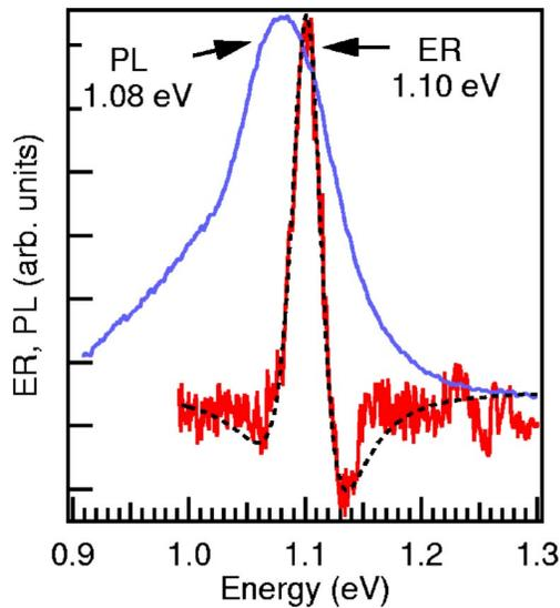
FIG. 1. Room temperature photoluminescence and electroreflectance spectra for  $\text{GaN}_{0.0085}\text{As}_{0.9775}\text{Bi}_{0.014}$  showing the optical band gap. The dotted line is a fit to the electroreflectance spectrum as discussed in Ref. 7.
