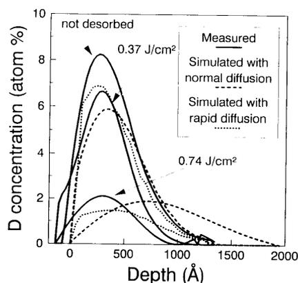
Fig. 2. Depth profile evolution after laser energy shot of  $0.37 \text{ J/cm}^2$  and energy ramp to  $0.74 \text{ J/cm}^2$ : experimental (—), and simulated with diffusion-limited (-----) and detrapping-limited (·····) processes. The Be sample was implanted at 1 keV with  $1.1 \times 10^{17} \text{ D/cm}^2$ .
