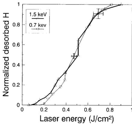
Fig. 4. Normalized hydrogen release after laser desorption from a Be sample implanted with two different energies of 0.7 keV (○) and 1.5 keV (△).
