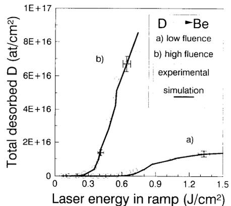
Fig. 1. Cumulative release of D implanted in Be after desorption by laser energy ramp: (a) 0.4 keV,  $1.75 \times 10^{16}$  D/cm<sup>2</sup>. (b) 1 keV,  $1.1 \times 10^{17}$  D/cm<sup>2</sup>.
