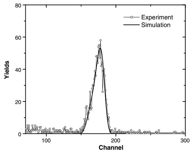
Fig. 3. NRA spectrum from 320 nm thick  $\text{GaAs}_{1-x}\text{N}_x$  film grown on GaAs wafer obtained using 3707 keV  $\text{He}^{2+}$  beam along with a SIMNRA simulation using the evaluated cross-sections.
