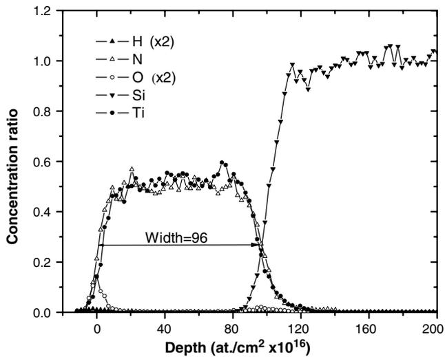
Fig. 1. Depth profile of the sample measured by ERD-TOF using 40 MeV  $\text{Cu}^{8+}$  beams, the element concentrations were normalized by Si signal.
